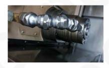
**Articulated Steel Tubes**, for the supply of coolant at low, medium or high-pressure. Also useful for air blasting operations. Ideal for both fixed-head and Swiss-type CNC lathes, vertical and horizontal machining centers, grinding or transfer machines.
